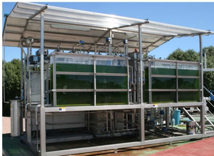
Figure 6.2. (A) Flow diagram of the MPBR pilot plant. Nomenclature: P: pump; DC: distribution chamber; PBR: photobioreactor; C: compressor; MT: membrane tank; WT: waste tank; and CIP: clean-in-place. (B) General view of the MPBR pilot plant.
