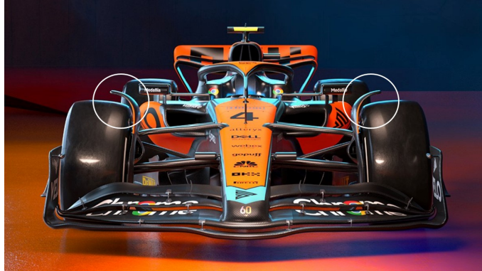
Figure 1.1: Image where upper wheel winglets can be easily seen on a F1 car [1]
