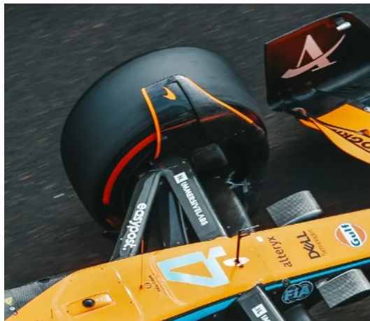
Figure 8.1: Slot left in the over-wheel winglet of the McLaren 2022 car [27]
