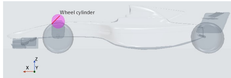
Figure 5.5: Over-wheel winglet block refinement area
