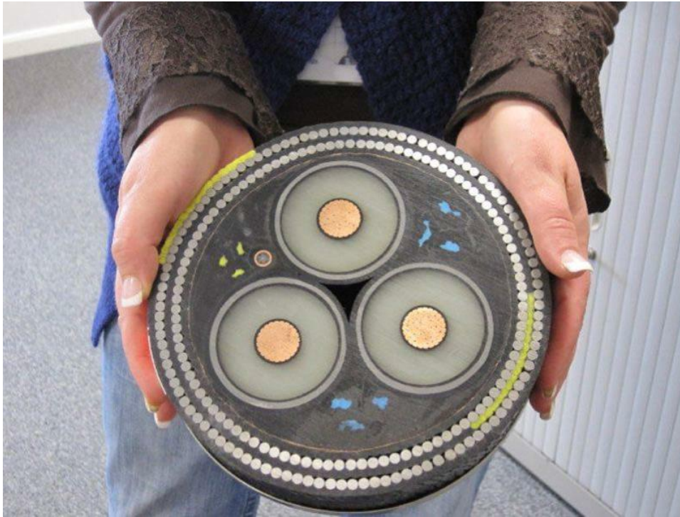
Figure 8: Offshore cable example
