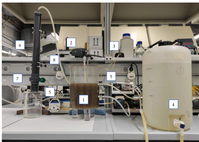
Figure 1. The outline of the experimental setup: (1) SBR (sequencing batch reactor); (2) stirrer; (3) air pump; (4) SW (synthetic wastewater) feed tank; (5) peristaltic pumps; (6) effluent sampling device; (7) removable screen; (8) timer outlet for the control of the sequencing phases in the SBR.
