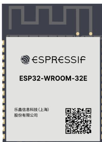
Figura 2: Microcontrolador ESP32-WROOM-32E.
