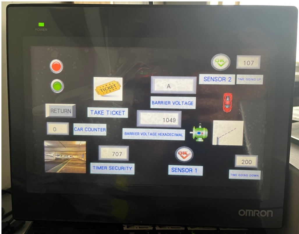
Fig. 3.41. High voltage adjustment, the barrier goes up and the motor rotates
