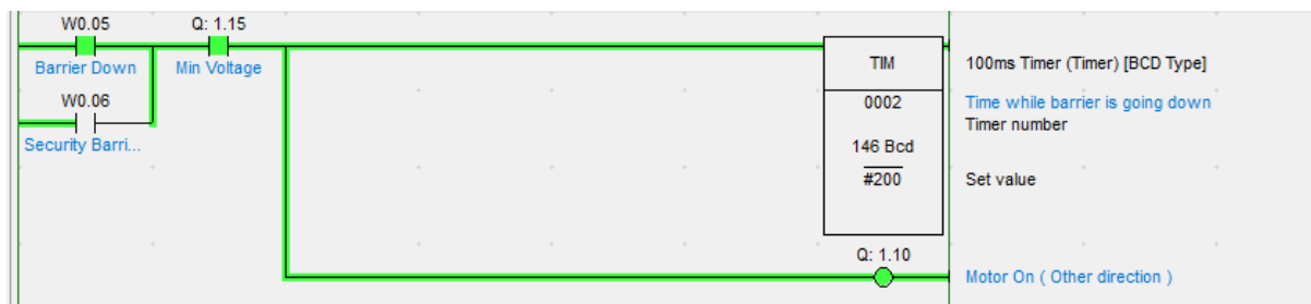
Fig. 3.22. Barrier is going down and the motor rotating
