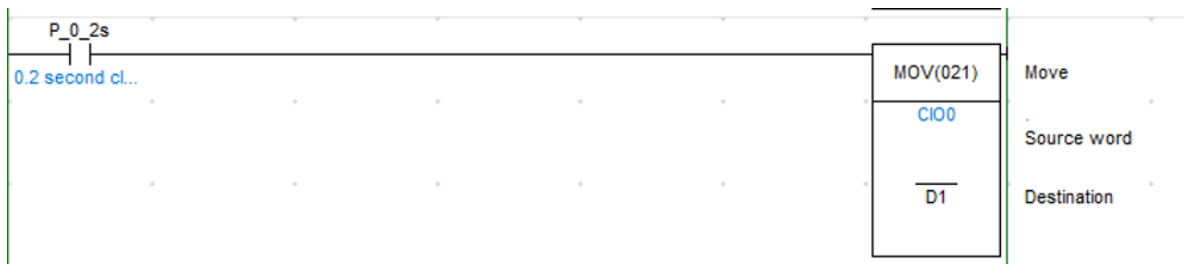
Fig. 3.6. Example of analog input with MOV(021) instruction
