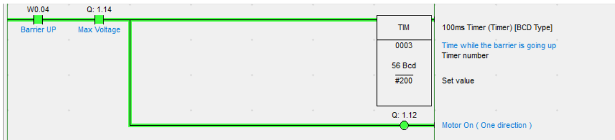
Fig. 3.20. The barrier is raising and the motor rotating
