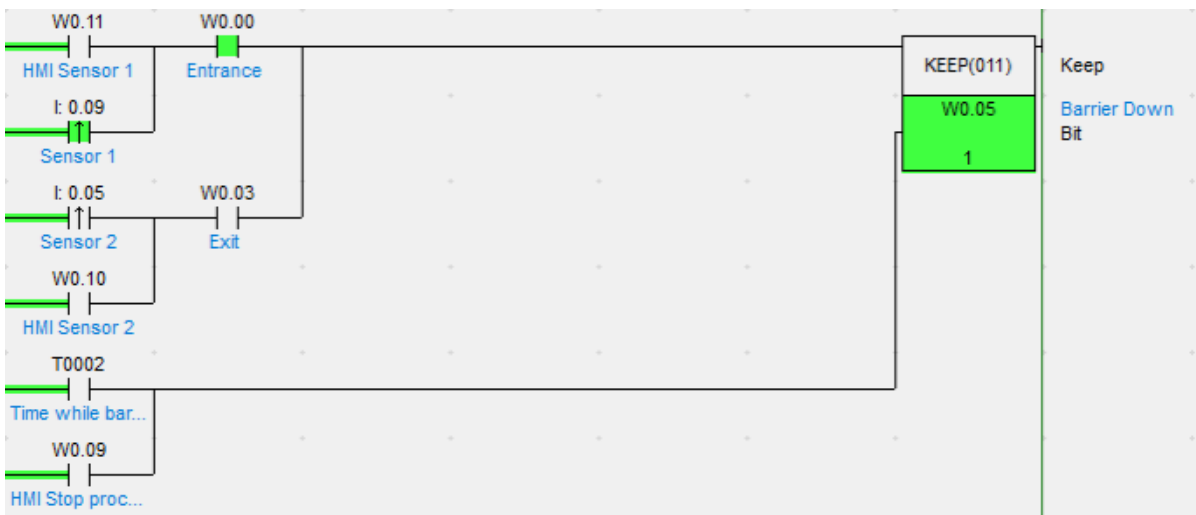
Fig. 3.21. Sensor 1 detects the car after it has gone through the barrier, and “Barrier Down” mode is activated
