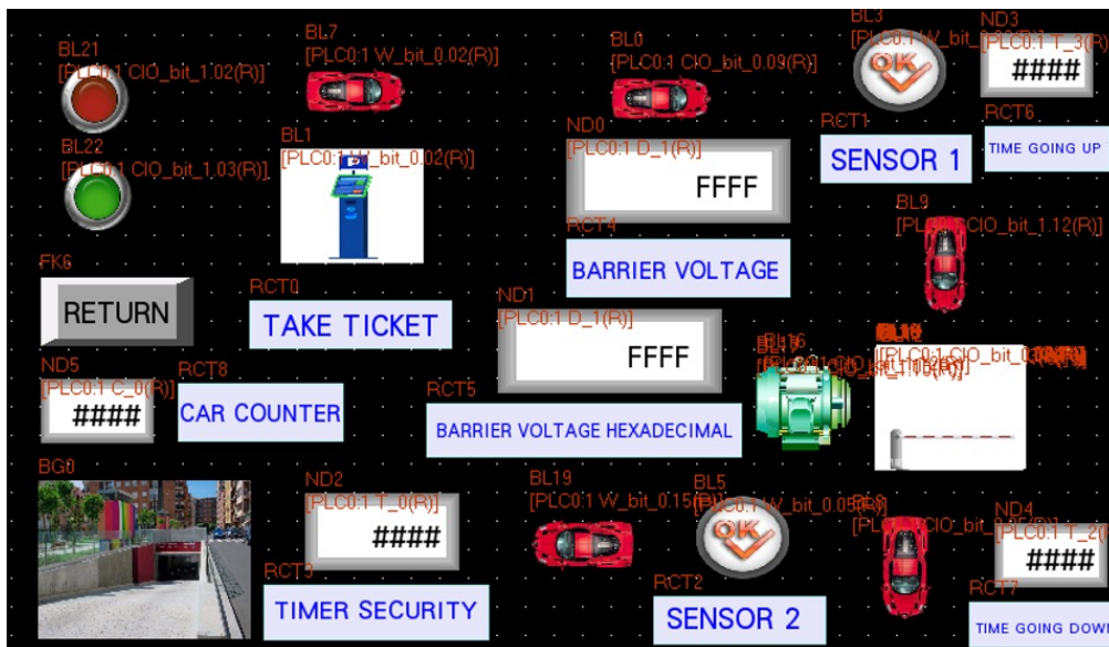
Fig. 3.45. Exit process with addressed I/O
