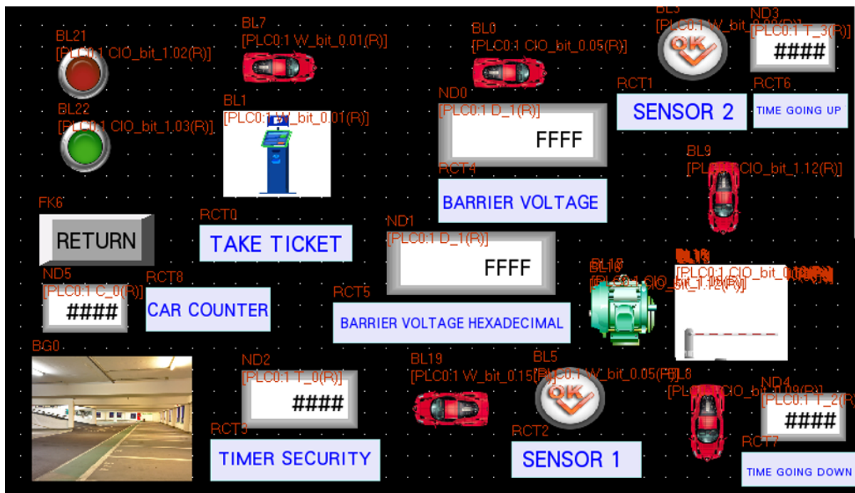
Fig. 3.37. Entrance process with addressed I/O
