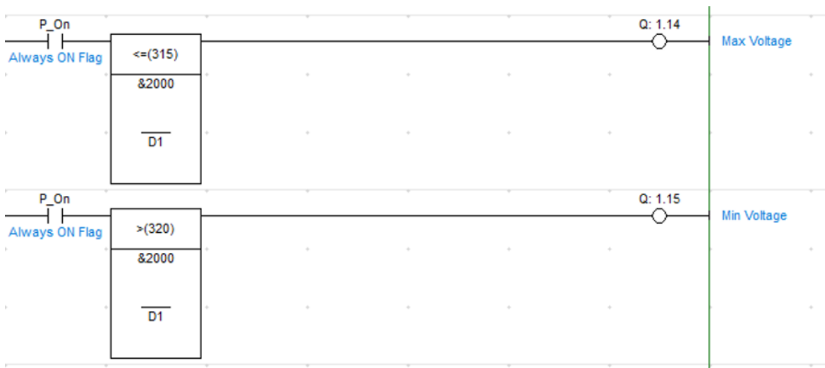
Fig. 3.7. Example of Analog Input with Comparison Instruction
