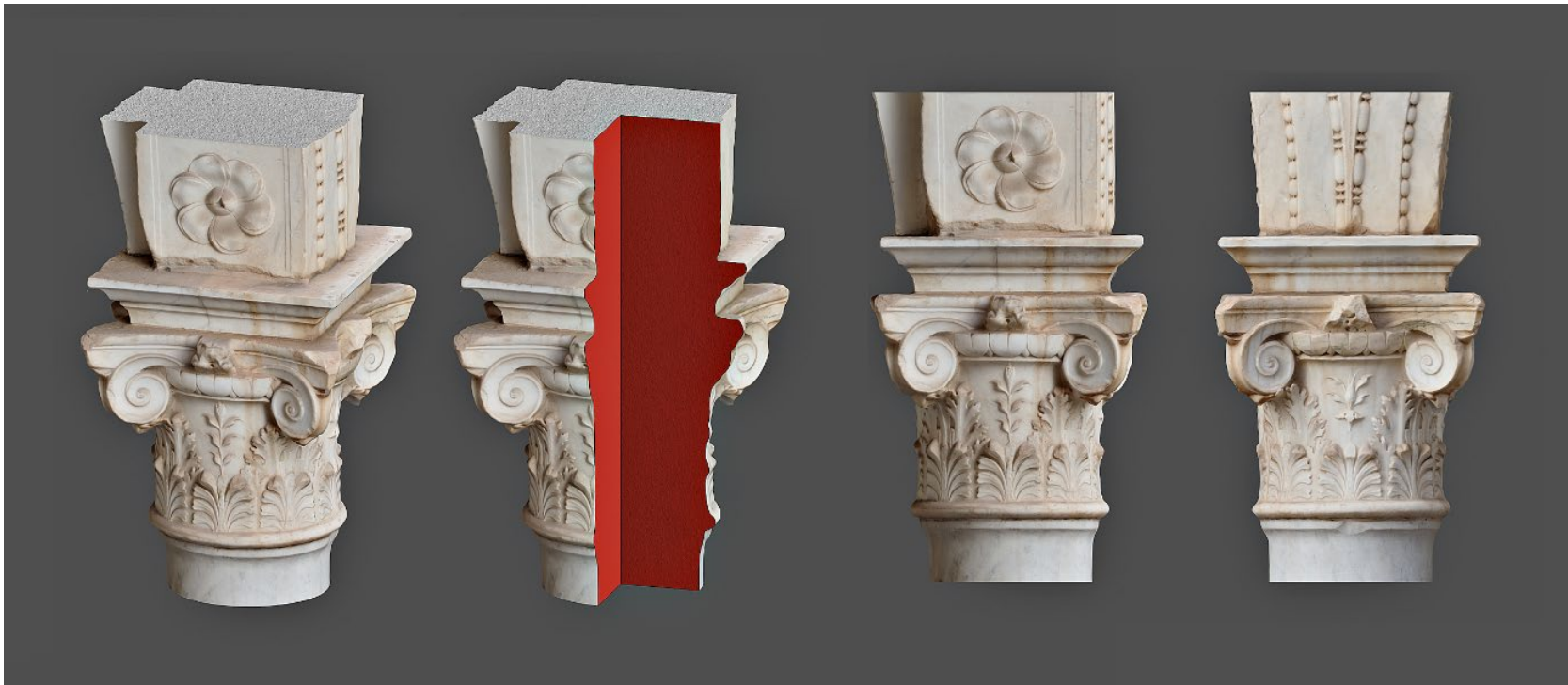
Fig. 15 - Resulting 3D model of the capital obtained from the photogrammetric survey.
