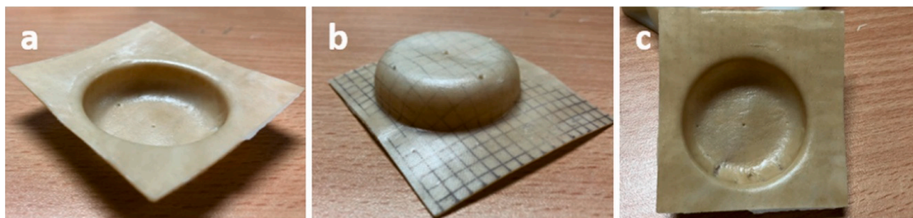
Fig. 4. Thermoformed tray based on poly(3-hydroxybutyrate) (PHB) reinforced with cellulosic rice husk fibers and compatibilized with hexamethylene diisocyanate (HMDDI): (a) bottom-side view, (b) top-side view and (c) bottom view. Reprinted from Sánchez-Safont et al. [106] under Creative Commons CC BY license.
