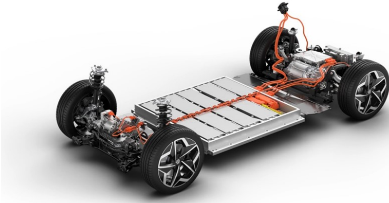
Figure 2–15: Battery electric vehicle skateboard architecture. (Adapted from [111])
