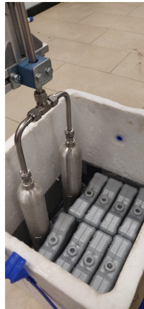
Figure 7: Sample cylinder submerged in glycol with PCMs.
