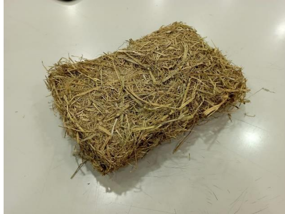
Figure 8. Rice straw insulation
