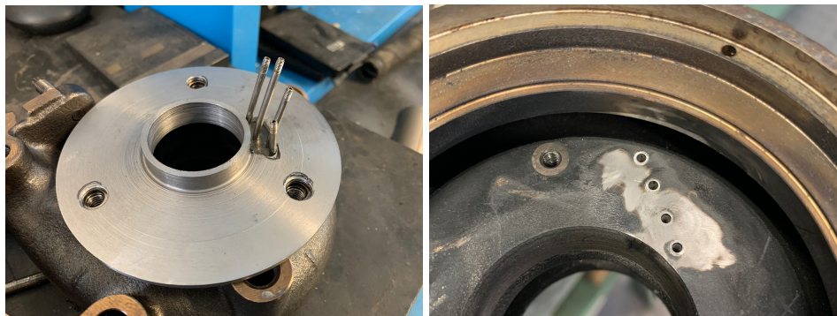
(a) External view of the pressure taps.
