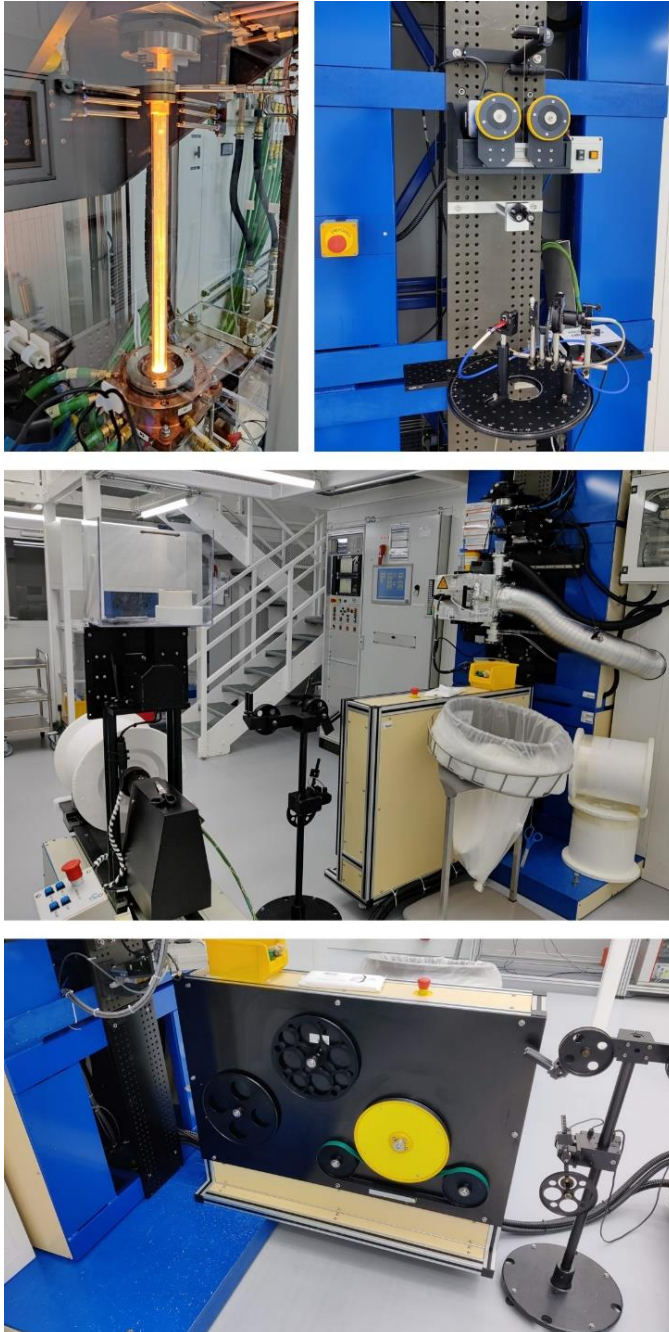
Fig. 5.12. (Top) From left to right, third and second floor of the fiber tower, respectively. The furnace locates at the third floor. (Middle) First floor of the fiber tower. (Bottom) Tractor system and spooling wheel.
