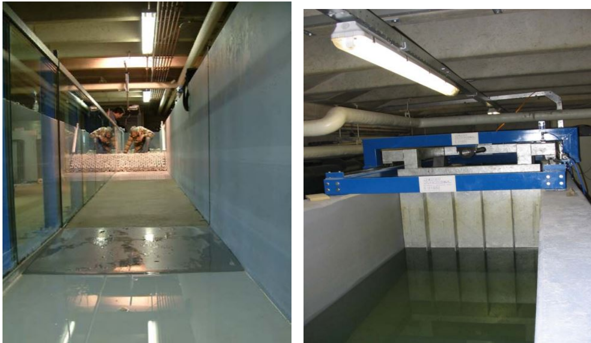
(a) The Large Wave Flume from inside
