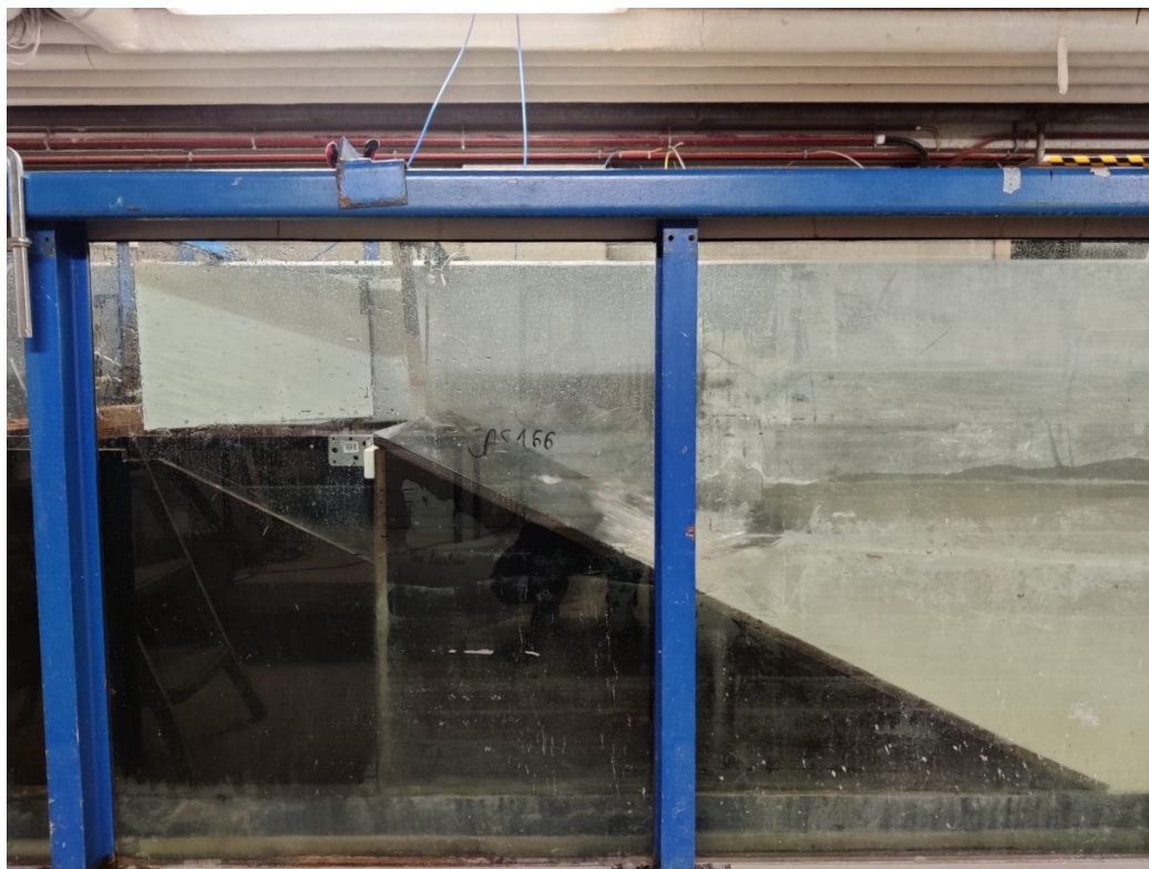
Figure 5.1: Model section with glass wall of the Large Wave Flume and geometry of the tested model during a test. Source: Chiara Ricci.
