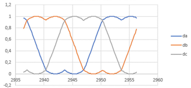
Fig. 5 Results of the duty cycle calculation for three-phase PWM and SVPWM. Calculated on-line at constant modulation index and frequency with the ESP32.
