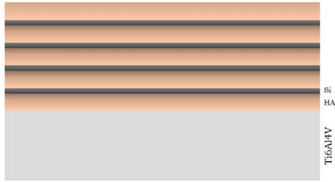
Fig. 1. Structural coating scheme.
