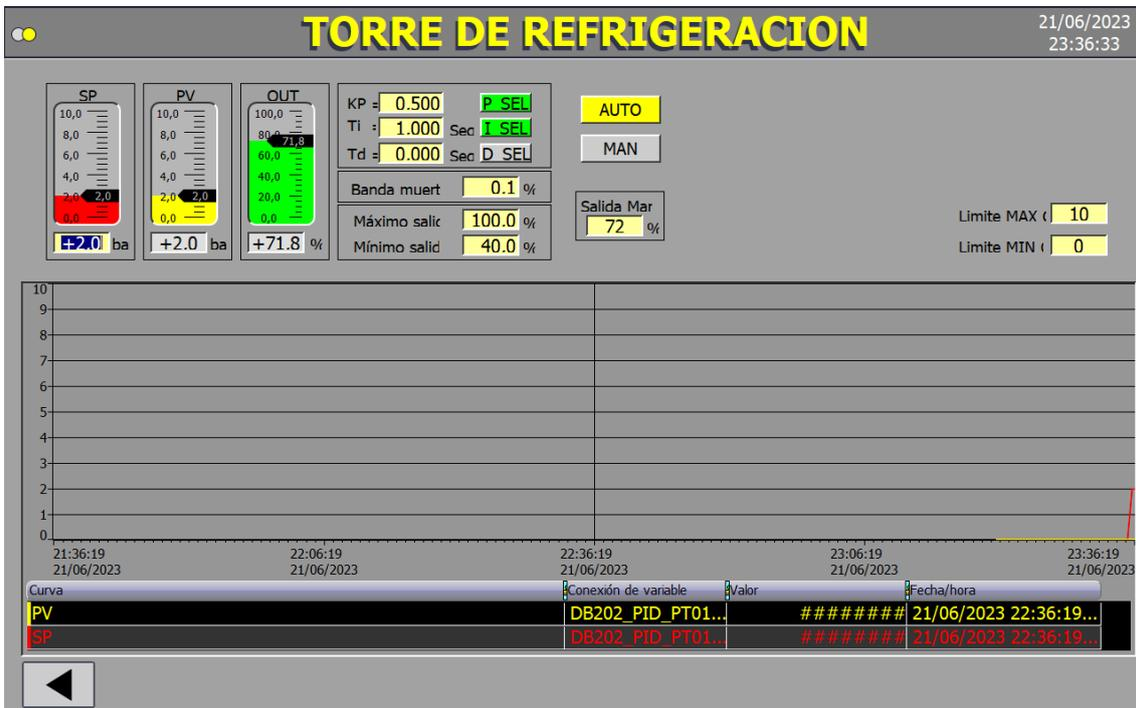
Figura 4. Pantalla PID HMI
