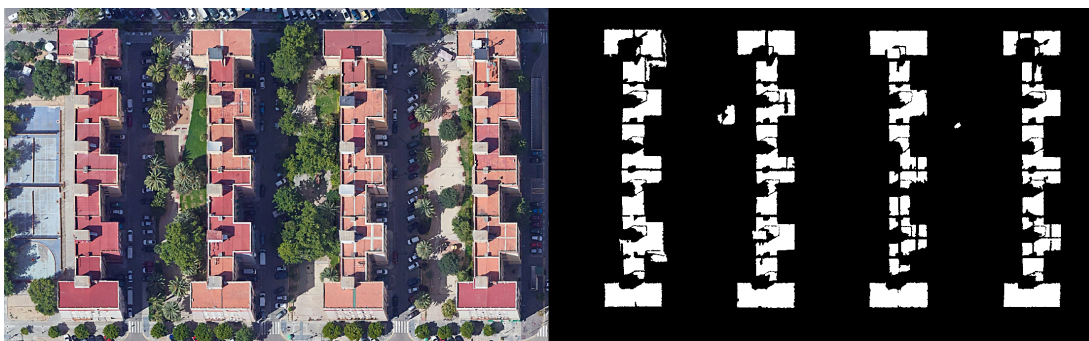
Figure 3.9: Fused mask for roof detection. The original image is shown (left) along the resulting mask (right). The mask aims to detect the flat roof RT, all the CRs have already been fused. Some blobs that do not belong to the roofs of the buildings have been selected but most of them will be erased in the next step. The left image is the cropped result of the GEP (LLC 2023) picture (2020) and the image on the right is produced using MATLAB (MathWorks 2022).
