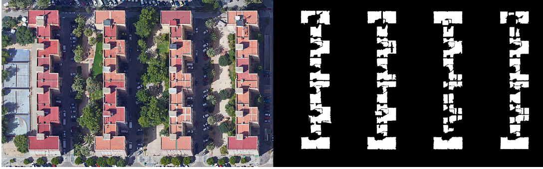
Figure 3.10: Manually cropped mask for roof detection. The original image is shown (left) along the resulting mask (right). There is a part of the building's facade in the left bottom part which is still included in the mask, but this part is visually undifferentiable from the roof, so, naturally, the AV algorithm fails. The left image is the cropped result of the GEP (LLC 2023) picture (2020) and the image on the right is produced using MATLAB (MathWorks 2022).
