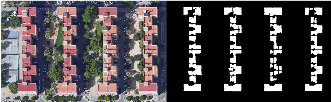
Figure 3.11: Final mask for roof detection. The original image is shown (left) along the resulting mask (right). The left image is the cropped result of the GEP (LLC 2023) picture (2020) and the image on the right is produced using MATLAB (MathWorks 2022).
