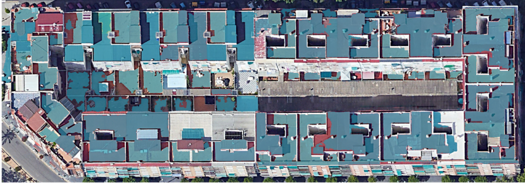
Figure A.8: Resulting mask of the eighth aerial image of the L'Illa Perduda neighbourhood. The original image is shown, and the resulting mask is overlapped onto it in a blueish colour. The base image is the cropped result of the GEP LLC 2023 picture (2020) and the overlapped mask is produced using MATLAB MathWorks 2022.
