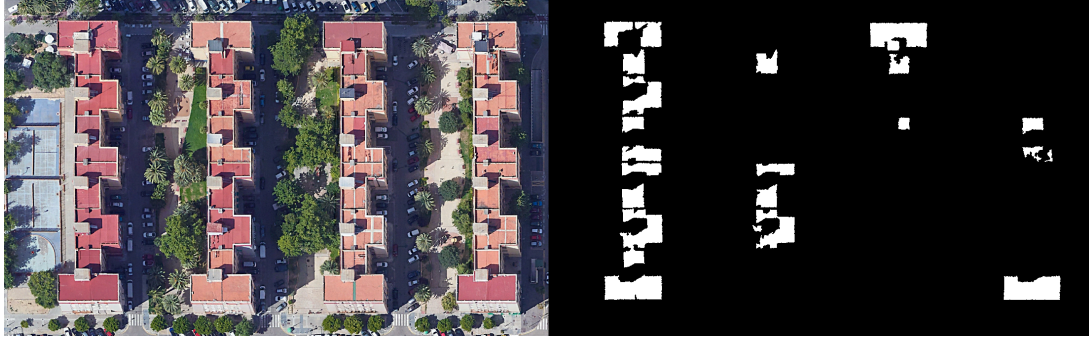
Figure 3.8: Filtered mask for roof detection. The original image is shown (left) along the resulting mask (right). The improvement from figure 3.7 is clear in cleaning selected points outside the building area and in polishing the detected surfaces. The left image is the cropped result of the GEP (LLC 2023) picture (2020) and the image on the right is produced using MATLAB (MathWorks 2022).
