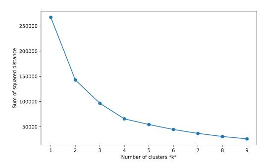
Figure 5.9: Elbow method visualization.
