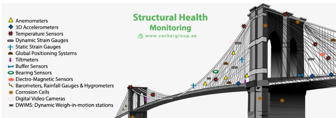
Figure 2: Example of sensors used in bridge SHM [6]
