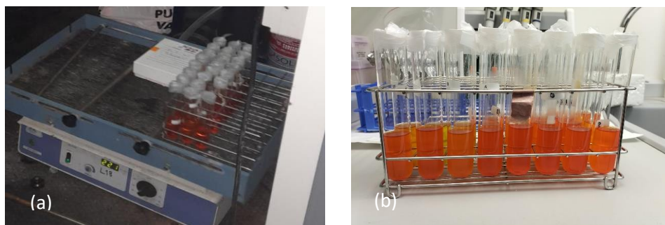
Figure 22. (a) Samples of pepper in the automatic shaker, (b) Extracted pepper samples for carotenoid determination.
