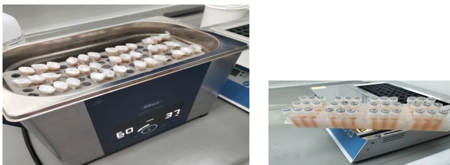
Figure 28. Samples of pepper in the ultrasonic bath under extraction hood.
