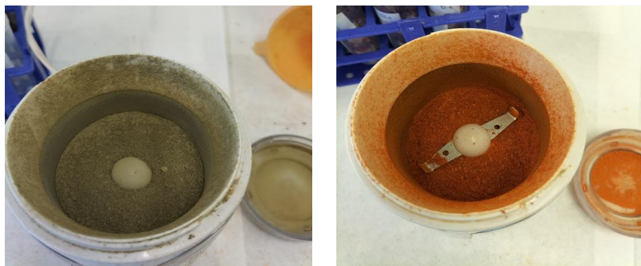
Figure 20. Sample grinding and preparation through coffee miller.
