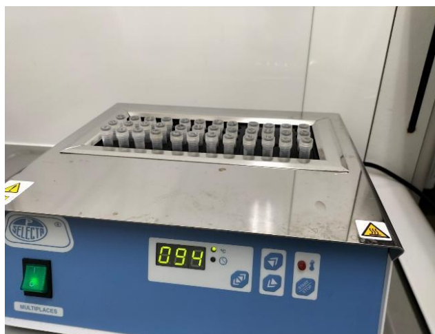
Figure 29. Hydrolysed samples in thermoblock.
