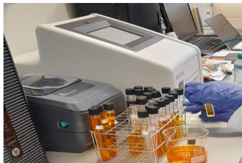
Figure 23. Spectrometric reading through BioTek instruments (EPOCH2TSC Agilent Technologies, USA).
