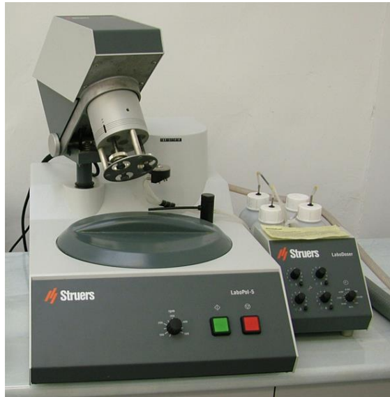
Figura 10: Pulidora LaboPol-5 y dosificador LaboDoser. (Budapest University of Technology and Economics)
