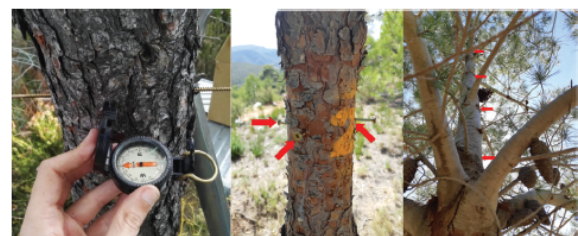
Figure 3. Electrode placement using a compass (left), identification of trees and radially location of the electrodes (center), electrodes separated longitudinally (right).
