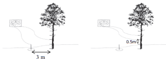
Figure 4. Electrode placement setup modes (left) measurements referenced to the ground, (right) bipolar setup.
