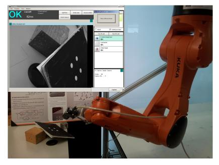
Figure 10. Setup used for the experiments: a 6R industrial robot with a camera mounted on the end-effector and a target that consists of a black square of side 300mm with four white points as visual features.
