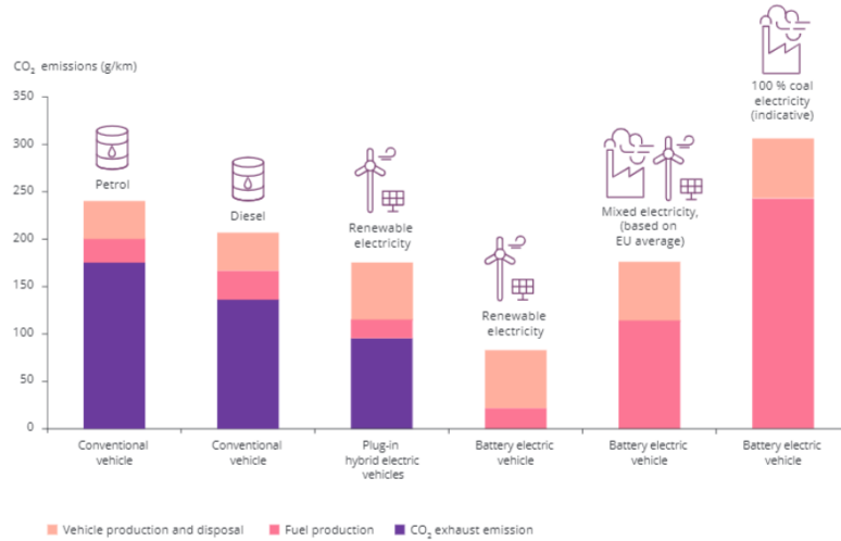
Figure 1.11. Comparison of CO 2 emissions for different powertrain typologies and energy sources. Source: EEA [33].
