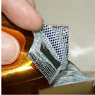
Figure 12: Multi-Layer Insulation Close-Up. [21]
