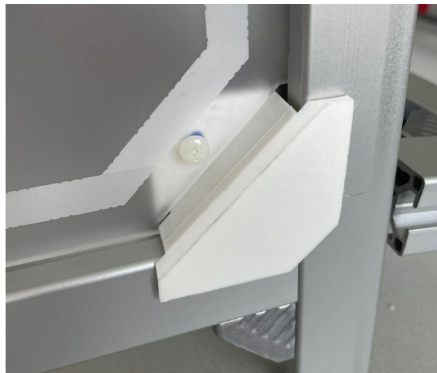
Figure 23 : Attachment Plexiglass – frame
