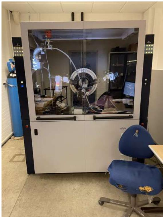
Figure 2.6: Bruker D8 Theta/Theta Goniometer used for XRD analysis
