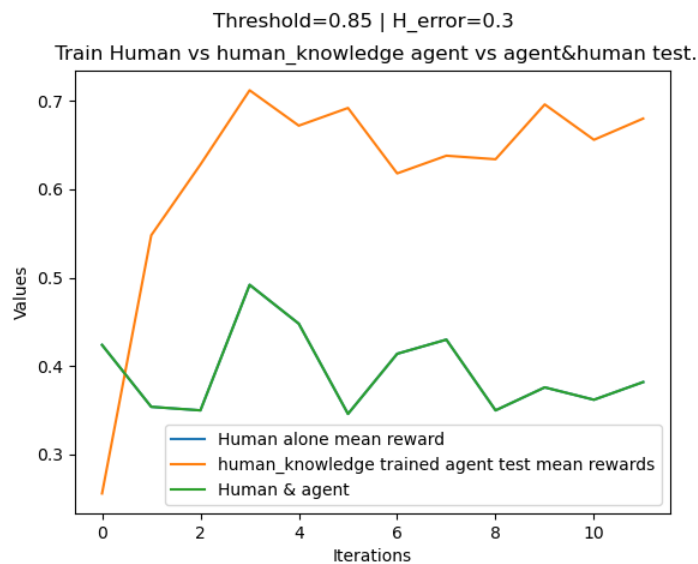
Figure 24. Example of wrong human assistance due to a high threshold. (y axe represents the mean reward values, x the iterations)
