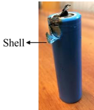
Figure 3-10: Broken canister/shell of a battery cell.
