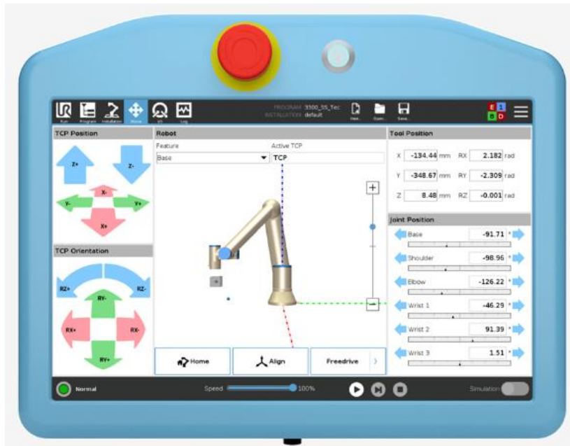
Figure 12. Control panel with touch screen, and graphical interface provided by Universal Robots for their cobots. Source: Do more than just keep up. Try our virtual simulator [69].
