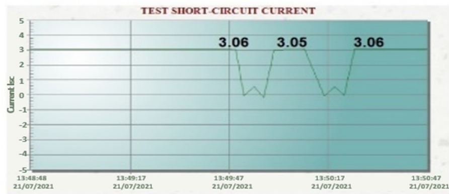
Figure 18. Voc test; (a) Voc test to the SP string; (b) Voc test to each one of the solar panels; (c) Isc test to each of the solar panels.
