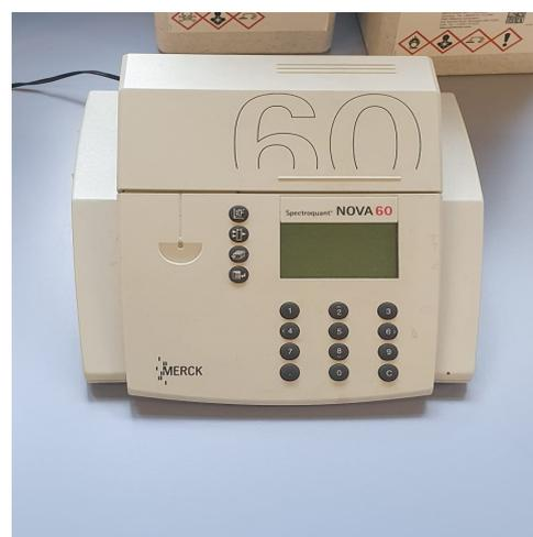
**(b)** Spectroquant photometer nova 60
