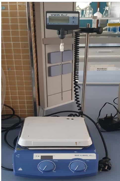
**Figura 3.8:** Placa Calefactora C-MAG HS 7
