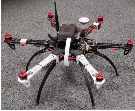
Figure 8.4: Hexacopter used in our experiments.
