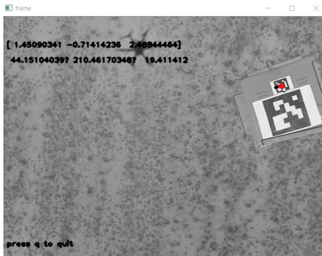
Figure 8.2: Image retrieved by the UAV camera after processing using OpenCV/ArUco libraries.
