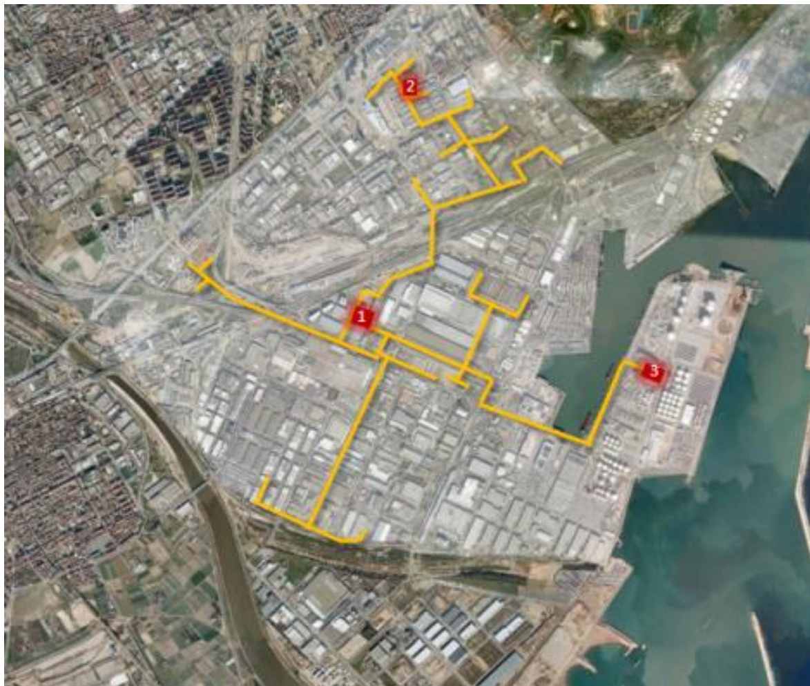
Figure 21. Phases of District Heating and Cooling Network Expansion in Barcelona. Source: Ecoenergies. (Elcacho, 2014)
