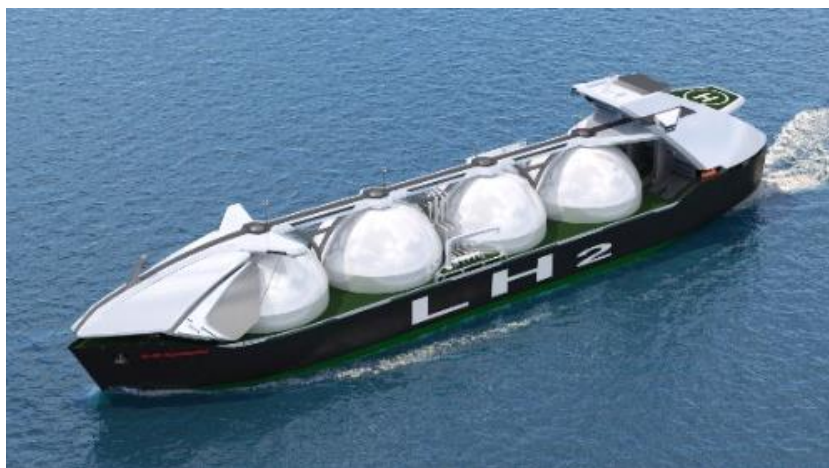
Figure 16. Simulated appearance of the completed 160,000\text{ m}^3 liquified hydrogen carrier [54]
