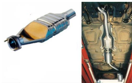
Fig. 3. Catalytic converter on a gasoline car. Source: Dieselnets technology guide.
