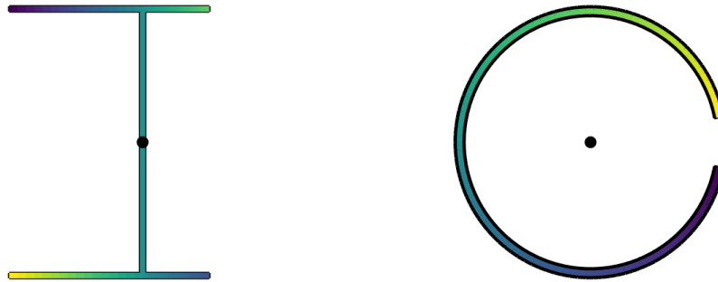
Fig. 3.34 Warping function for open cross-section beams. (Left) I-shape cross-section, (right) C-shape cross-section.
