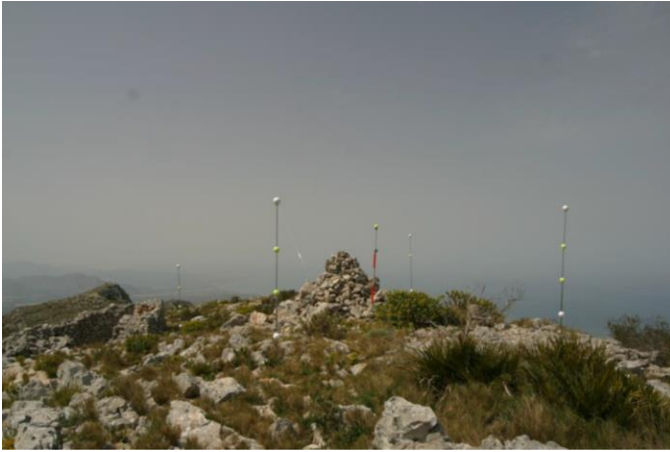
382 Fig. 4. MONGO. The pole with a yellow ball on its end (center of the image) marks the position from the initial 383 set of coordinates. (Image by Luis García-Asenjo.)
