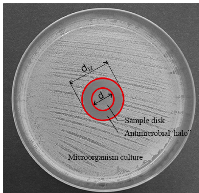
Fig. 16. Normalized width of the antimicrobial “halo” of a scaffold calculated by the inhibition zone ( d_{iz} ) and the scaffold diameter ( d ). Reprinted by kind permission of ref. [410]. Copyright 2018 MyJoVE Corporation.
