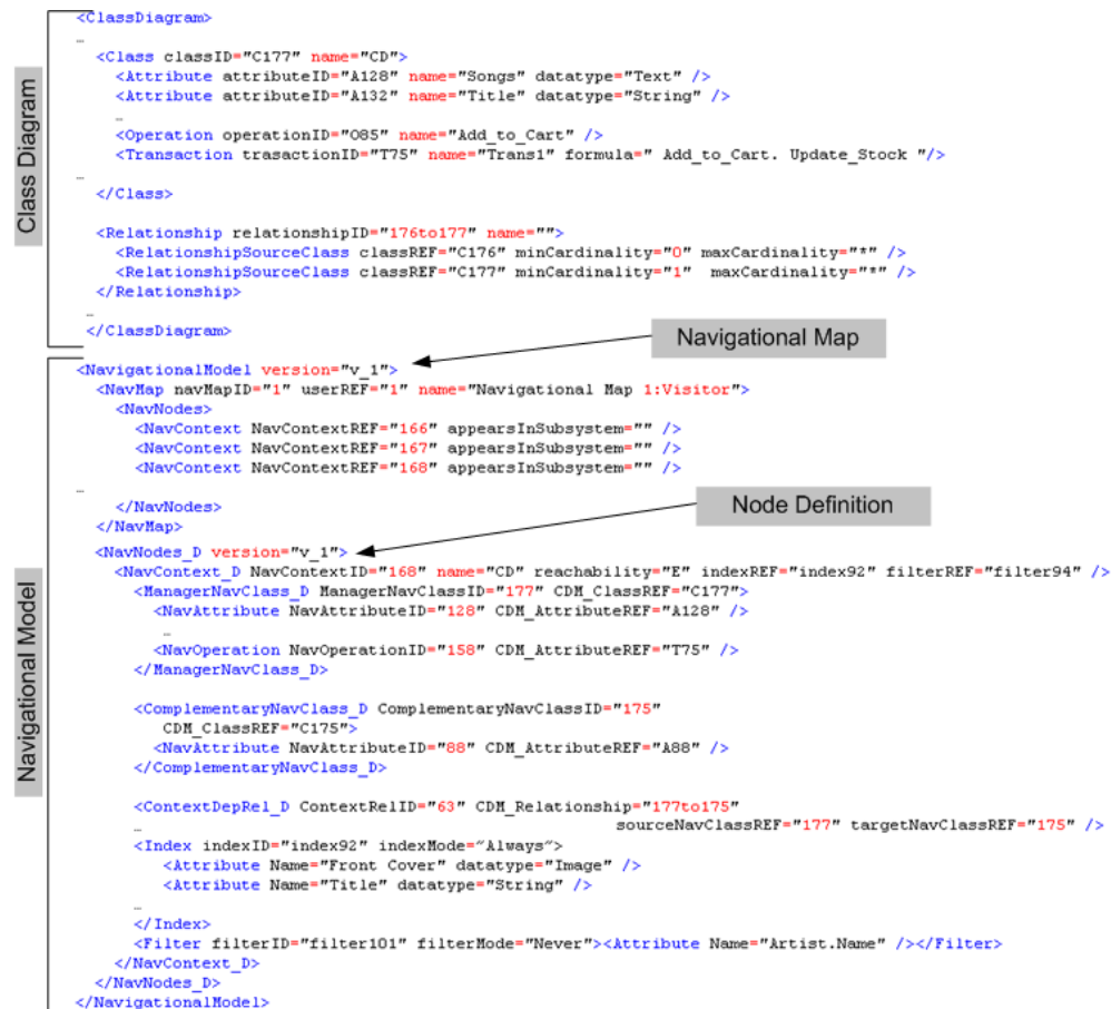
Figure B9 Example of XML code for storing OOWS models
