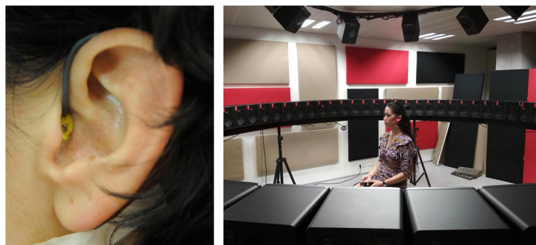
Fig. 1 Example of BRIR measurement and microphone inside the ear detail
