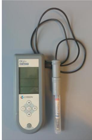
Figura 8. Conductímetro Crison CM35 +
