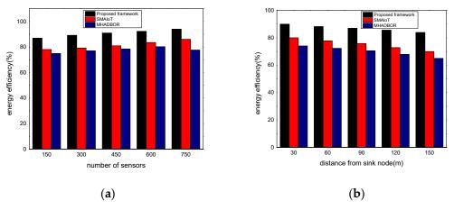
Figure 8. (a) Energy efficiency with varying sensors and (b) Energy efficiency with varying distance.
