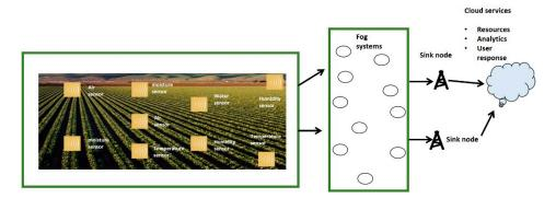
Figure 1. Scenario for fog-based IoT agricultural system.
