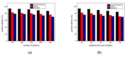
Figure 6. (a) Packets delivery with varying sensors and (b) Packets delivery with varying distance.
