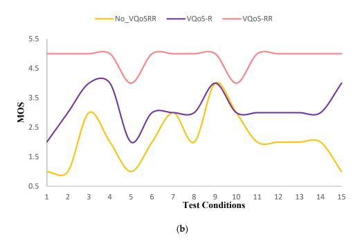
Figure 12. The MOS values of the tested videos. (a) SD resolution; (b) HD resolution.
