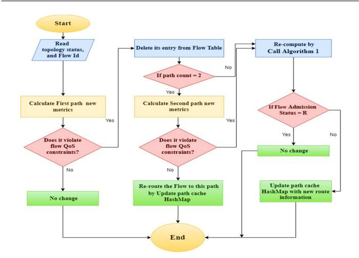
Figure 2. Dynamic re-routing algorithm (DR-RA) flowchart.
