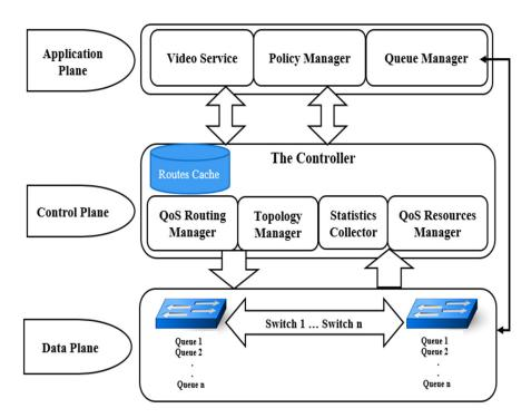
Figure 1. The VQoSRR SDN architecture.
