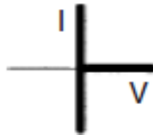
Figure 9. MOSFET quadrant operation. Carries in one direction or blocks in both directions.
