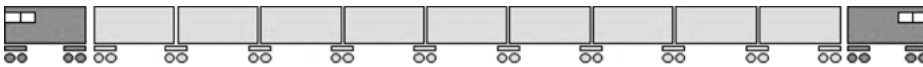
Fig. 13: Scheme of an articulated train with two power cars and nine passenger cars.
