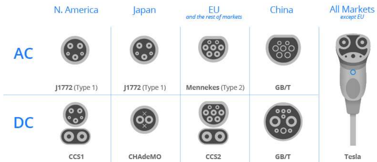
Figure 2: Comparison of EV charging connectors by region and current type [9].
