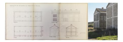
Figure 2. Plan of the prototypes of the "Torres de la Serna" tobacco drying sheds (1962. ACMAPAMA. INC Project. Photograph: Authors 2017
