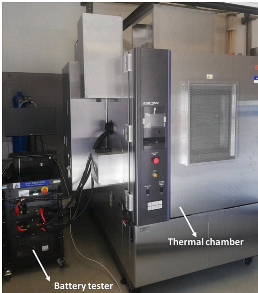
Fig. 1. Test bench for battery cell characterization.
